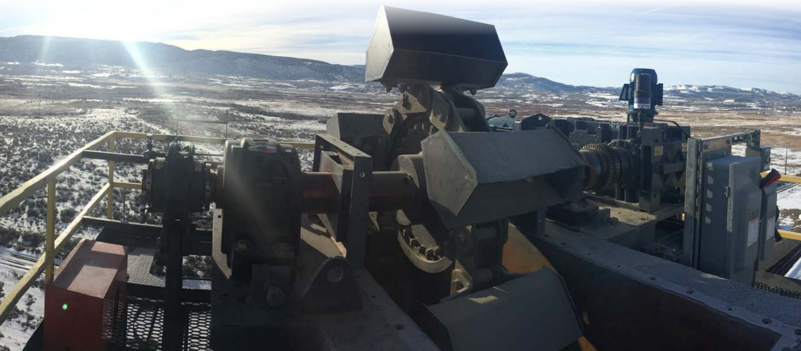
Segmental rim traction wheel on cement and aggregate application
