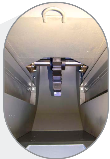
Curved bottom plate in the boot section
