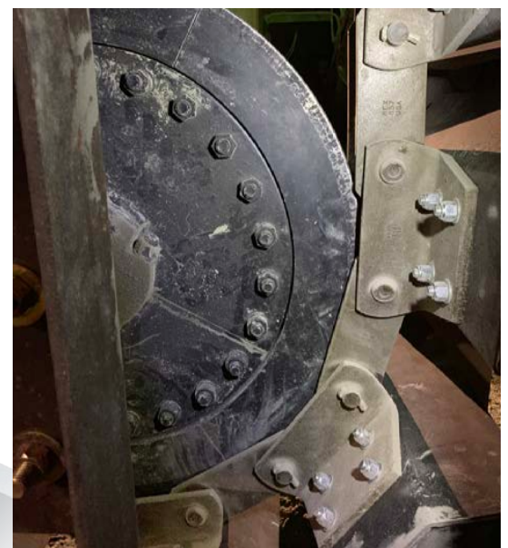
Segmental traction wheel with split hub
